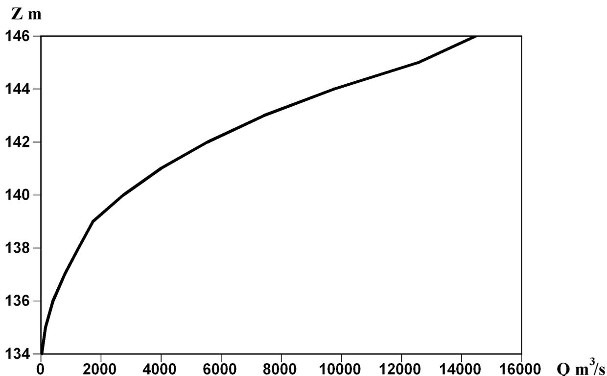
Fig. 5a. Discharge - stage curve for the paleochannel of pra-Seim River near Kudintsevo, calculated with Chezy-Manning formula.
