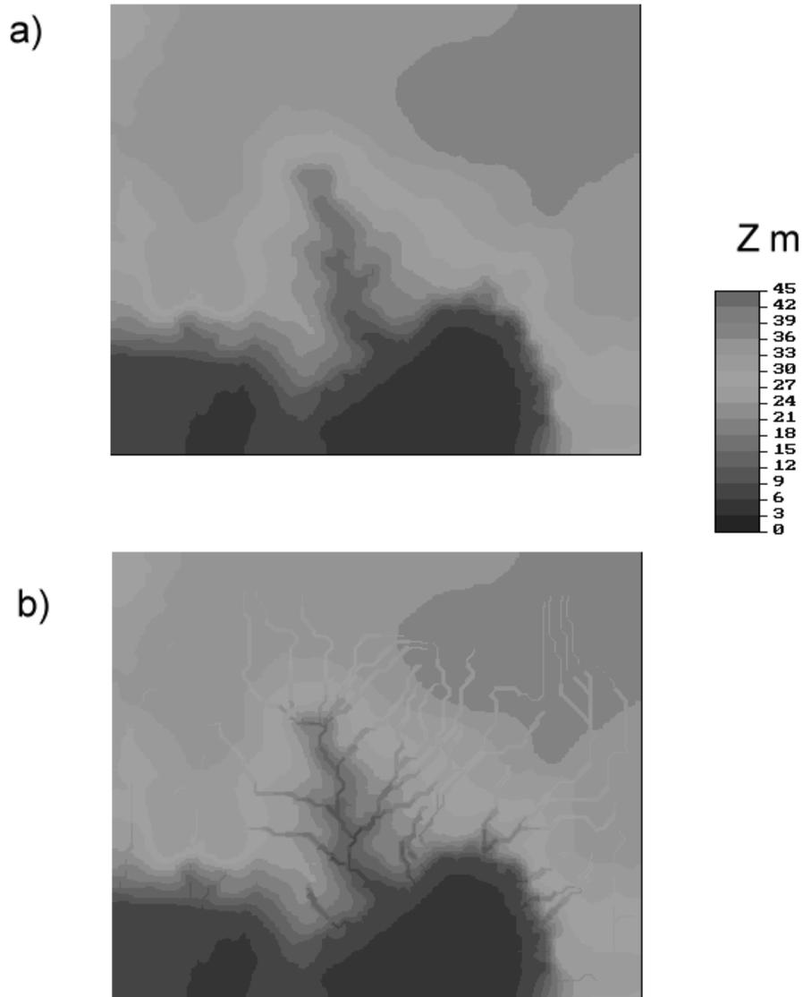
Fig.3 Effect of land conservation on gully erosion. a) Initial terrain in 1986 before exploitation camp building and in the condition of thaw water drainage or vegetation cover recultivation.; b) gully growth in the condition of thaw water increase and vegetation cover deterioration.
