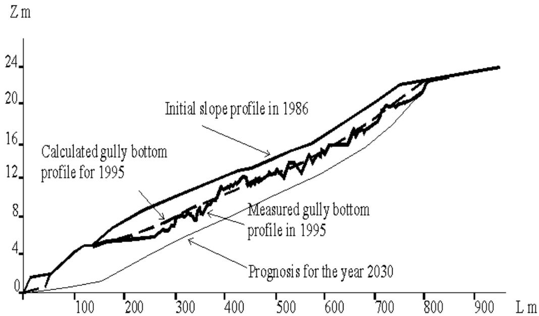
. Dynamic gully erosion model verification: case study of longitudinal profile evolution and prediction for the gully on the Yamal Peninsula (Russia)
